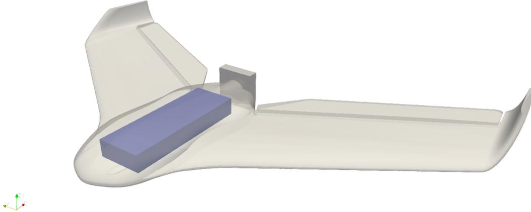
Figure 6: Physical space constraints handled by the projection parametrizer.
