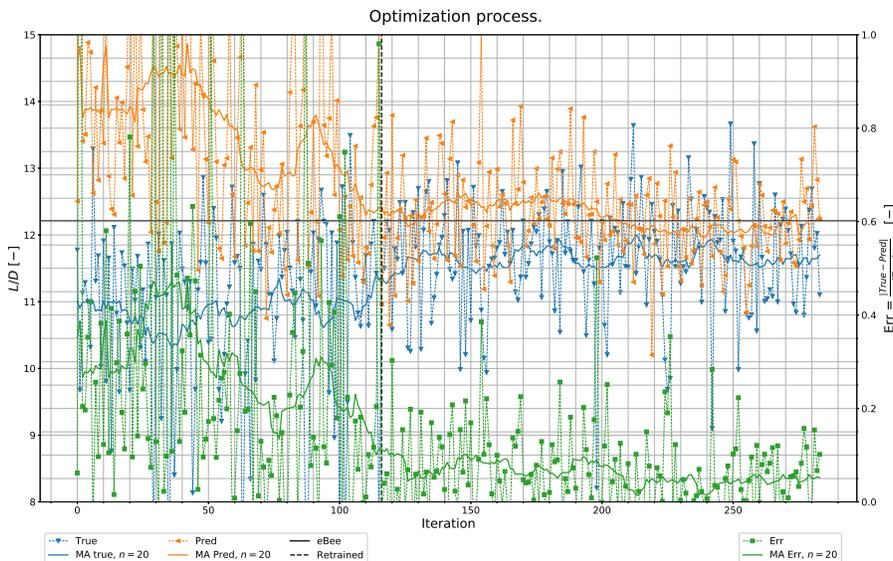
Figure 8: Evolution of the objective over the optimization process.
