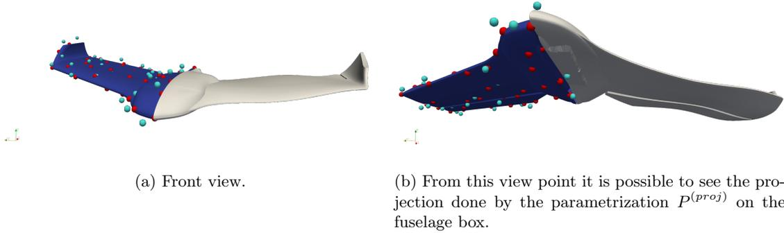
Figure 5: Reference geometry (blue) and a random configuration. Control points  $\mathbf{C}$  (red) and deformed control points  $\mathbf{C} + \mathbf{D}$  (light blue).
