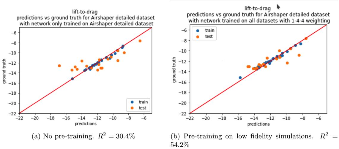
Figure 9: Predictions of L/D ratio on high-fidelity simulations for a model trained on high-fidelity simulations where: (a) The model was trained directly on 50 high-fidelity simulations. (b) The model was pre-trained before on low-fidelity ones. We can see that pre-training the network between fine-tuning it brings a substantial improvement (more than 20%) in  $R^2$  error, which motivates the transfer-learning approach.
