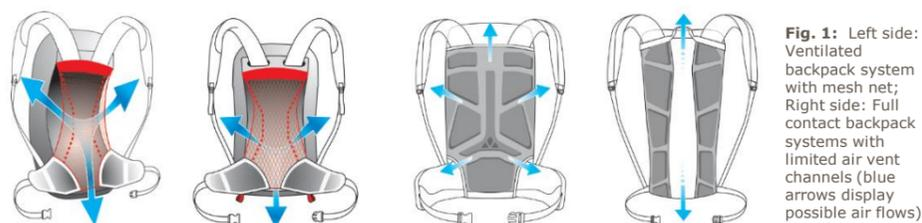
**Fig. 1:** Left side: Ventilated backpack system with mesh net; Right side: Full contact backpack systems with limited air vent channels (blue arrows display possible air flows)
