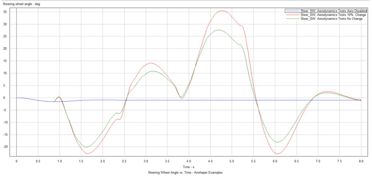
Figure 15: Steer angle versus time for different aero conditions
