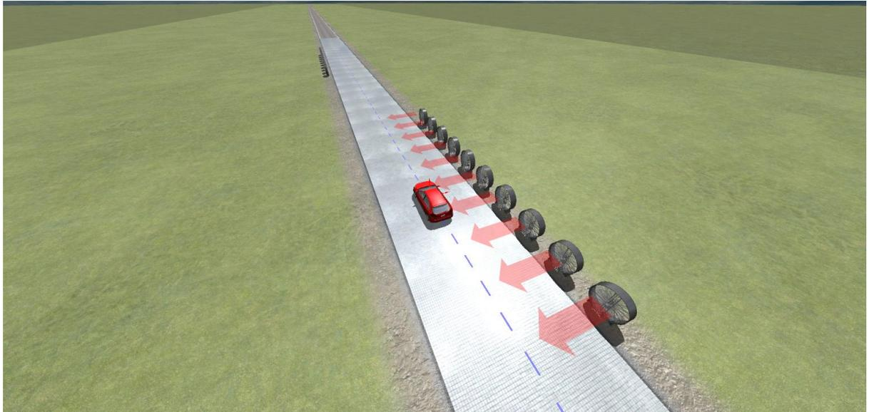
*Figure 22: Crosswind Procedure setup*
