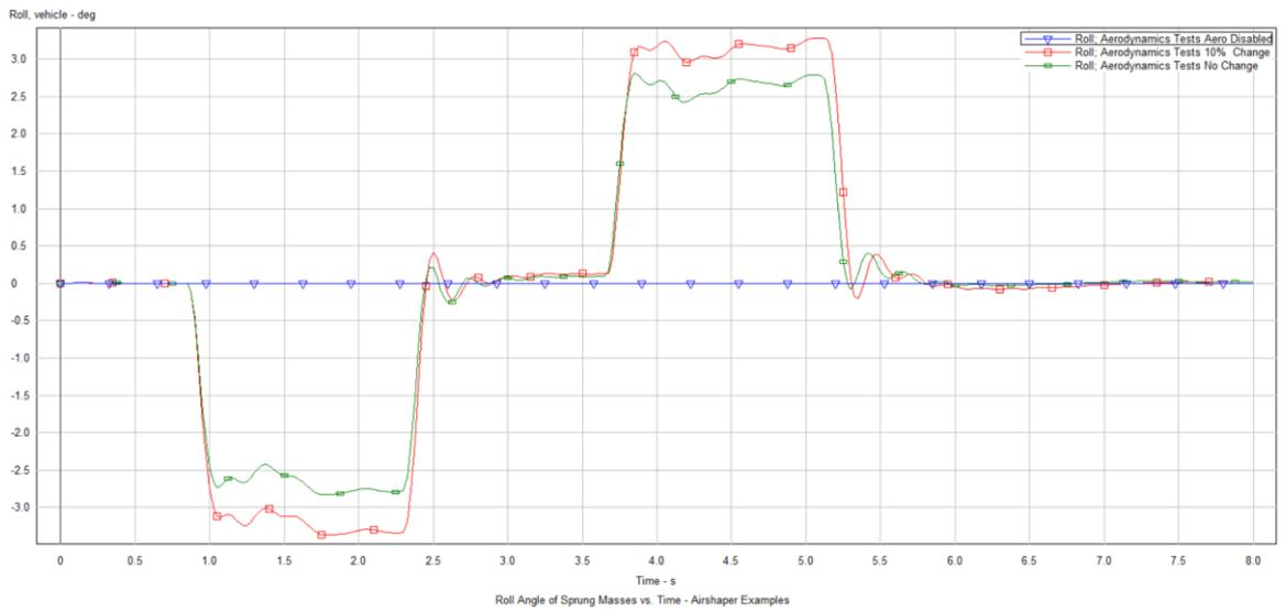
Figure 17: Roll angle versus time for different aero conditions
