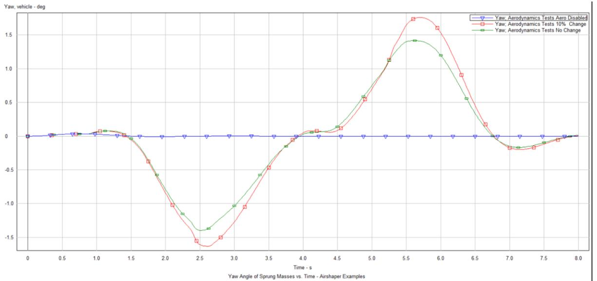
Figure 16: Yaw angle versus time for different aero conditions
