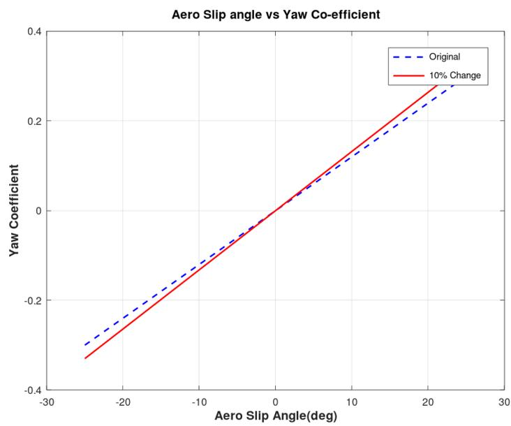
Figure 32: Aero Slip versus yaw co-efficient
