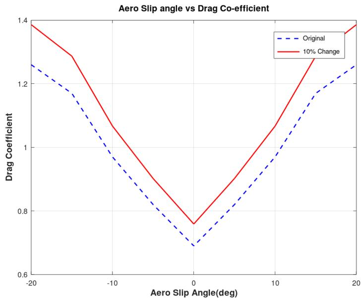
Figure 37: Aero Slip versus drag co-efficient
