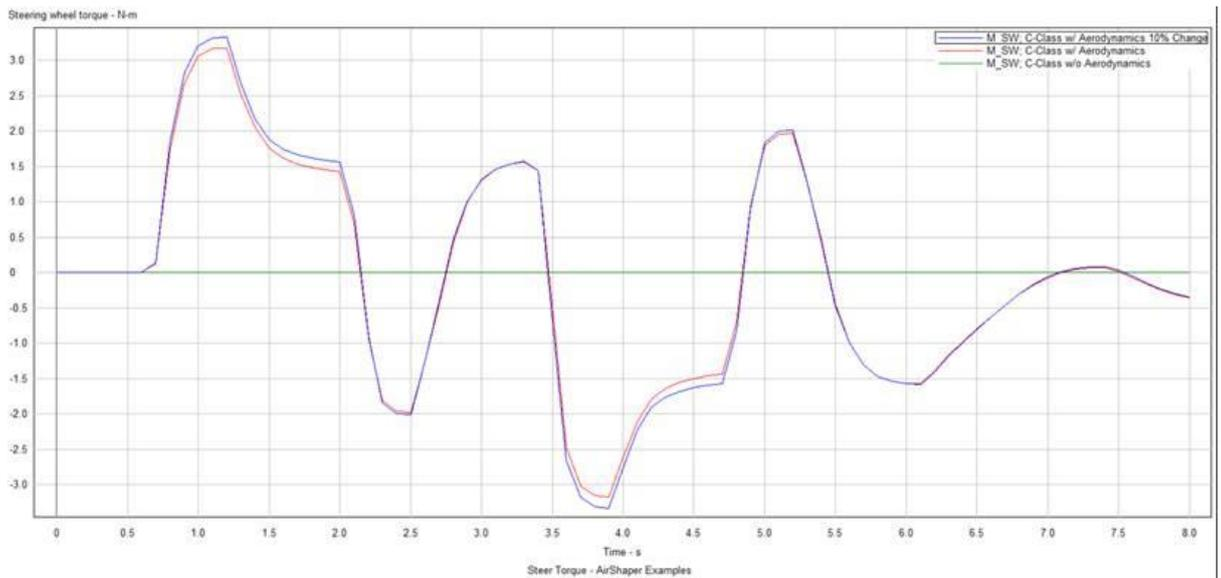
Figure 11: Steering Torque v/s time comparison crosswind only lateral coefficients changed
