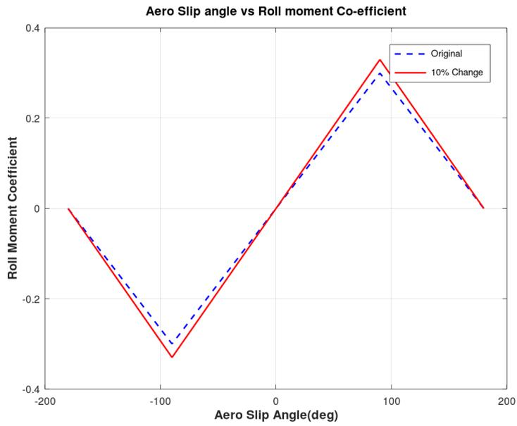
*Figure 27: Roll Moment versus Aero slip*
