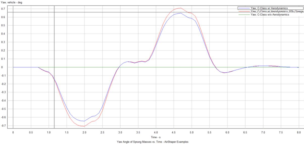
Figure 4: Yaw angle deviation due to crosswinds all coefficients changed
