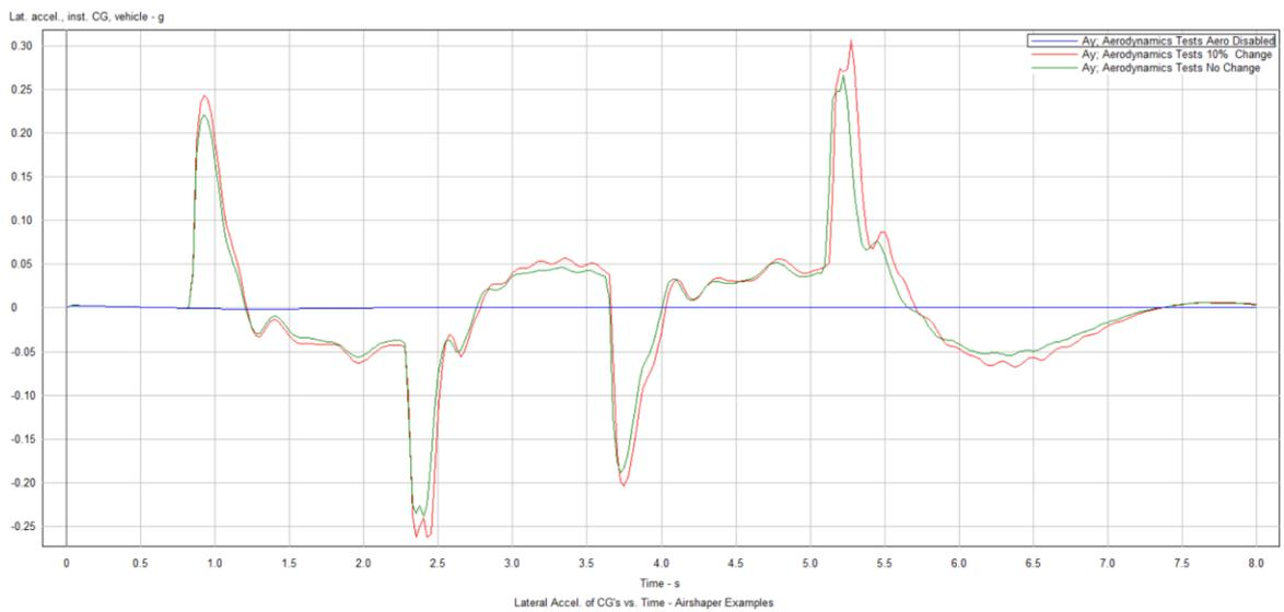
Figure 18 : Lateral acceleration versus time for different aero conditions
