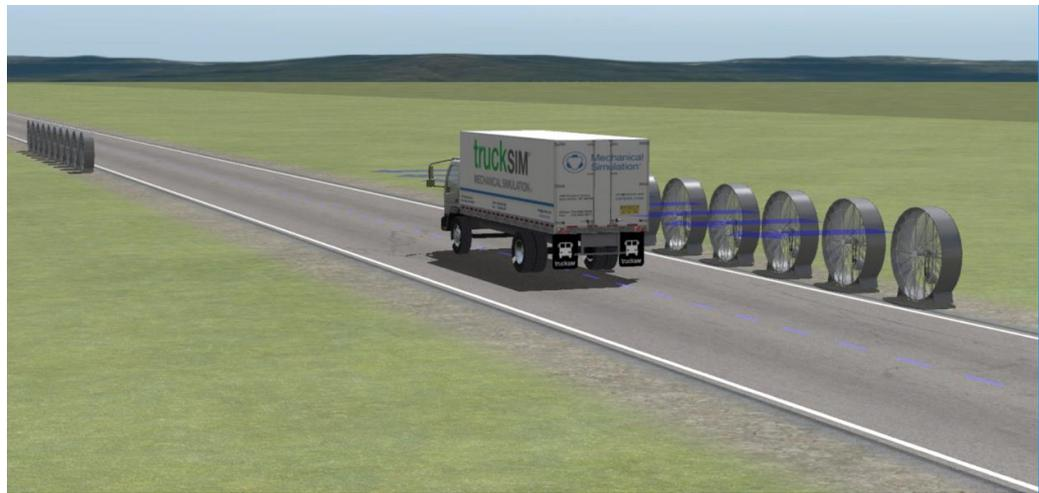
*Figure 14: TruckSim Crosswind Simulation*
