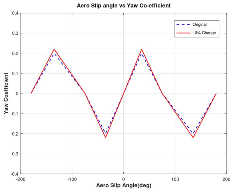
Figure 25: Yaw coefficient versus Aero Slip Angle
