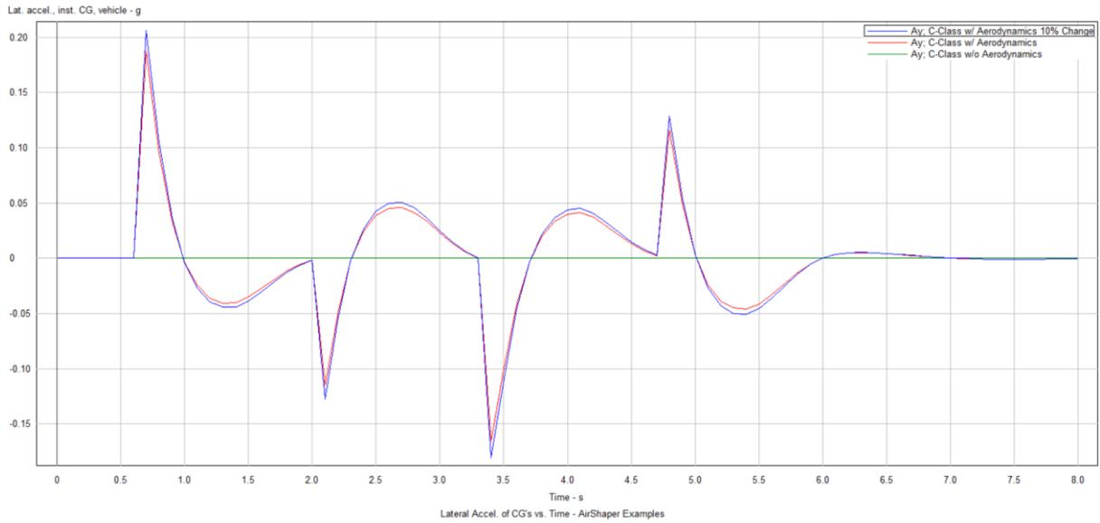
Figure 8: Lateral Acceleration comparison crosswind all co-efficient changed
