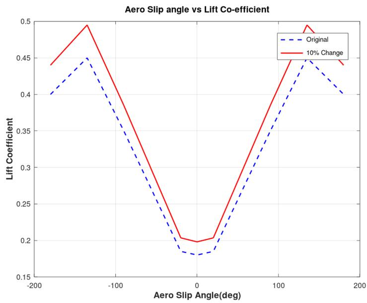
*Figure 28: Lift Coefficient versus Aero Slip*
