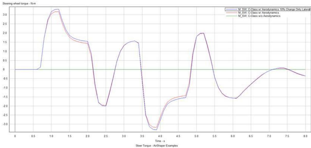
Figure 10: Steering Torque v/s time comparison crosswind all co-efficient changed
