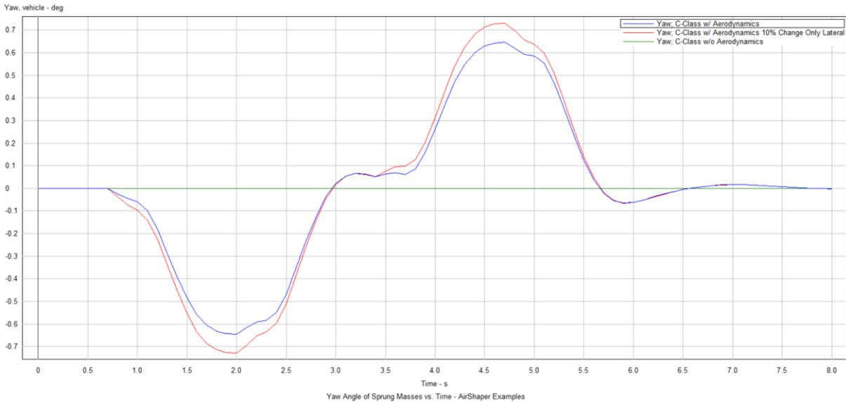
Figure 5: Yaw angle comparison crosswind only lateral coefficients changed
