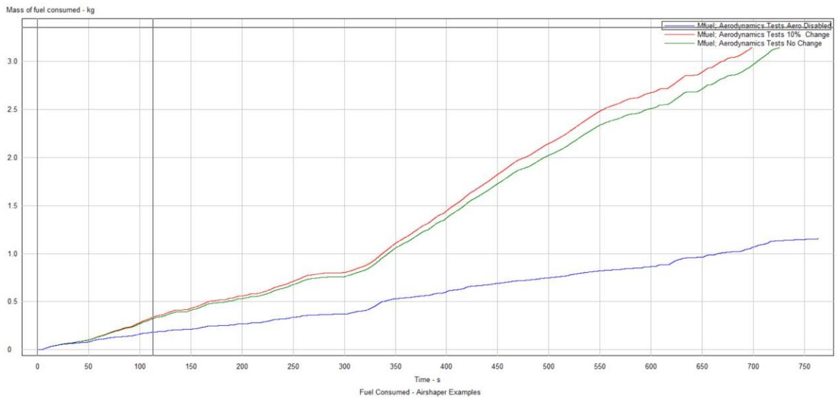
Figure 21 : Fuel Consumption over EPA Highway cycle
