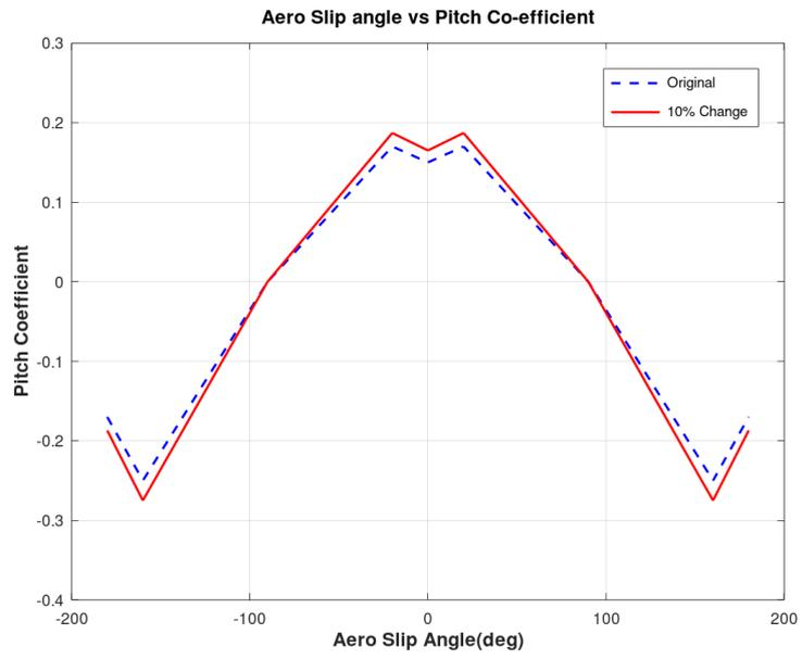
Figure 26: Pitch coefficient versus Aero Slip
