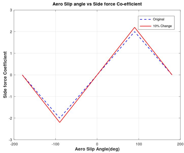
Figure 29: Side force coefficient versus Aero Slip
