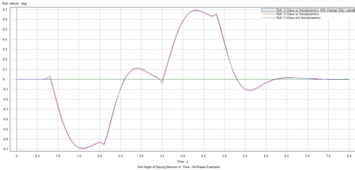
Figure 7: Roll angle variation due to Crosswinds all lateral coefficients changed
