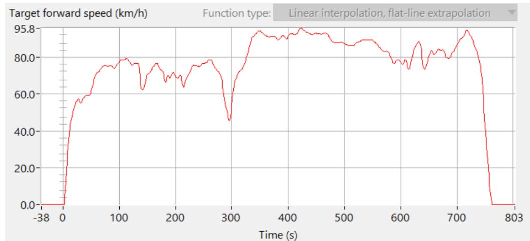
Figure 20: Vehicle Speed profile EPA Highway cycle
