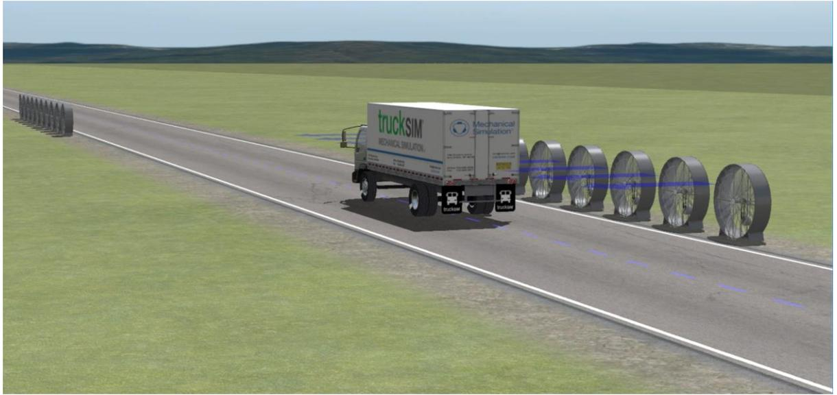
Figure 31: TruckSim Crosswind Simulation
