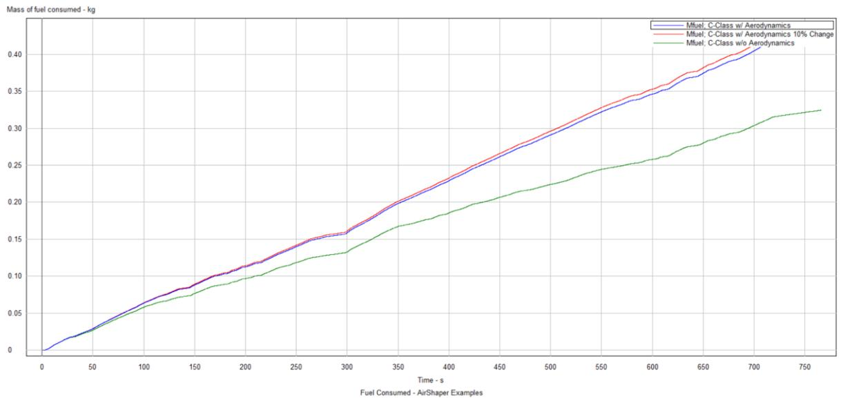
Figure 13: Fuel Consumed Over EPA Highway Cycle
