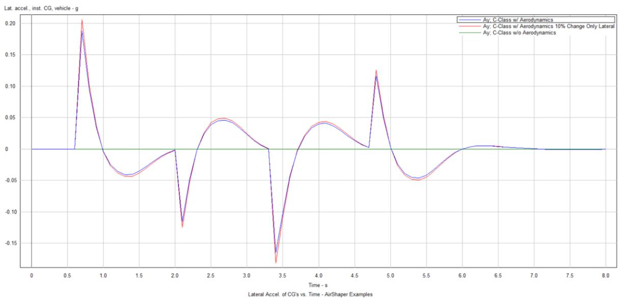
Figure 9: Lateral Acceleration comparison crosswind only lateral coefficients changed
