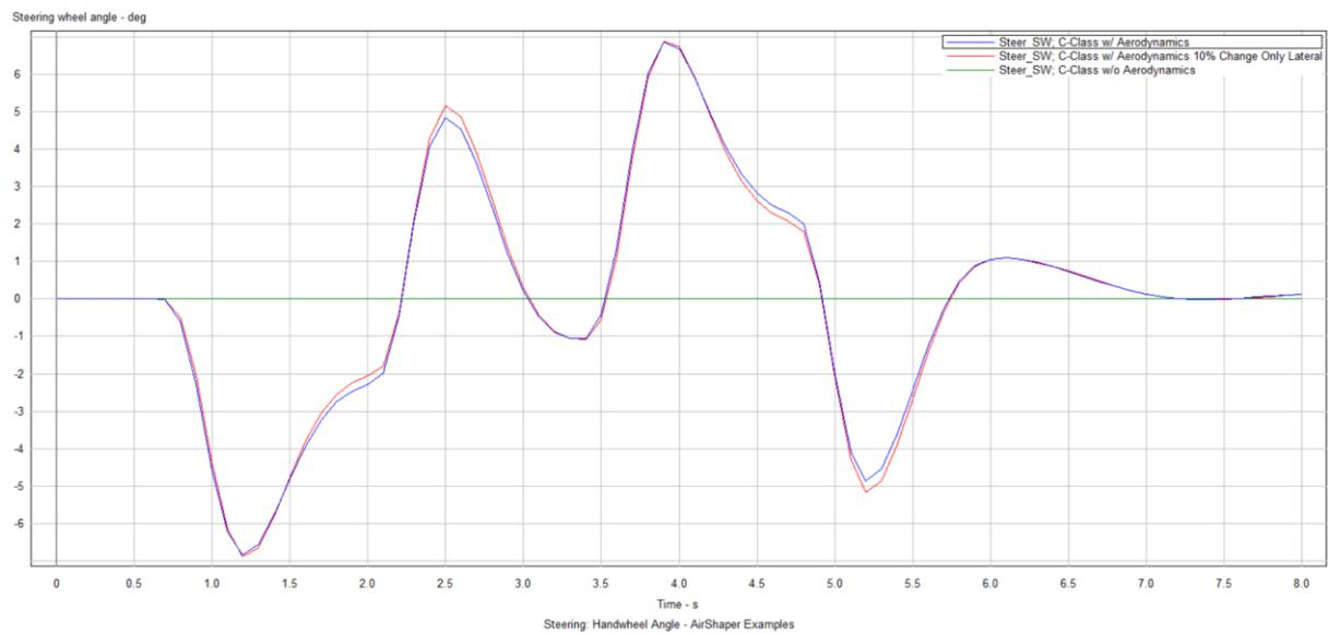
Figure 3: Steering wheel angle deviation due to crosswind only lateral coefficient changed
