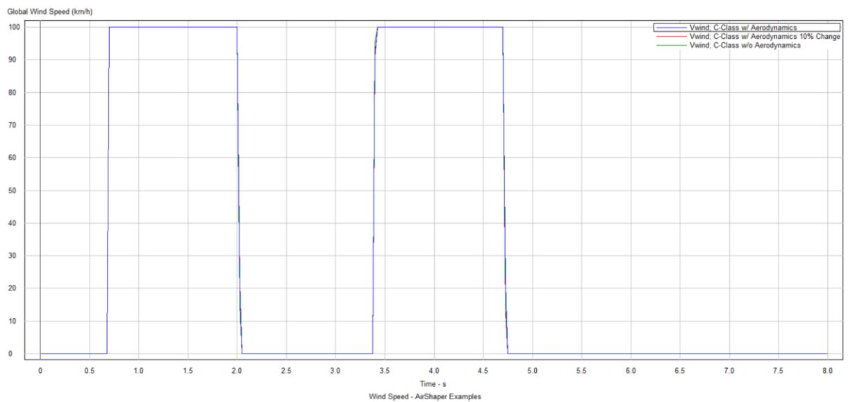
*Figure 23: Crosswind velocity inputs 100kmph*
