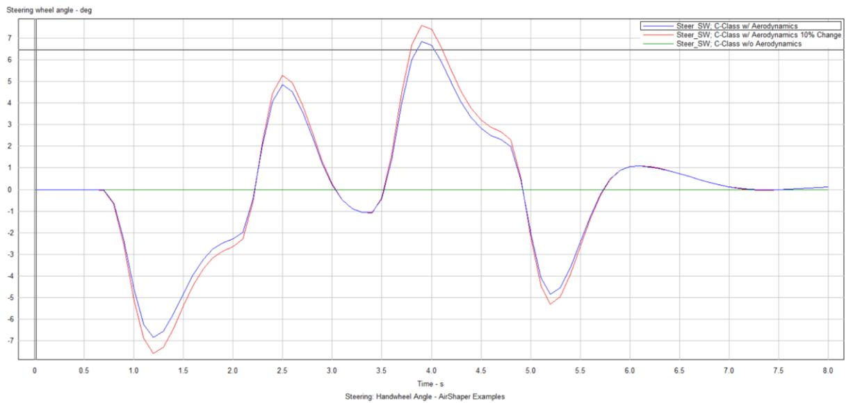
Figure 2: Steering wheel angle deviation due to crosswinds all coefficients changed
