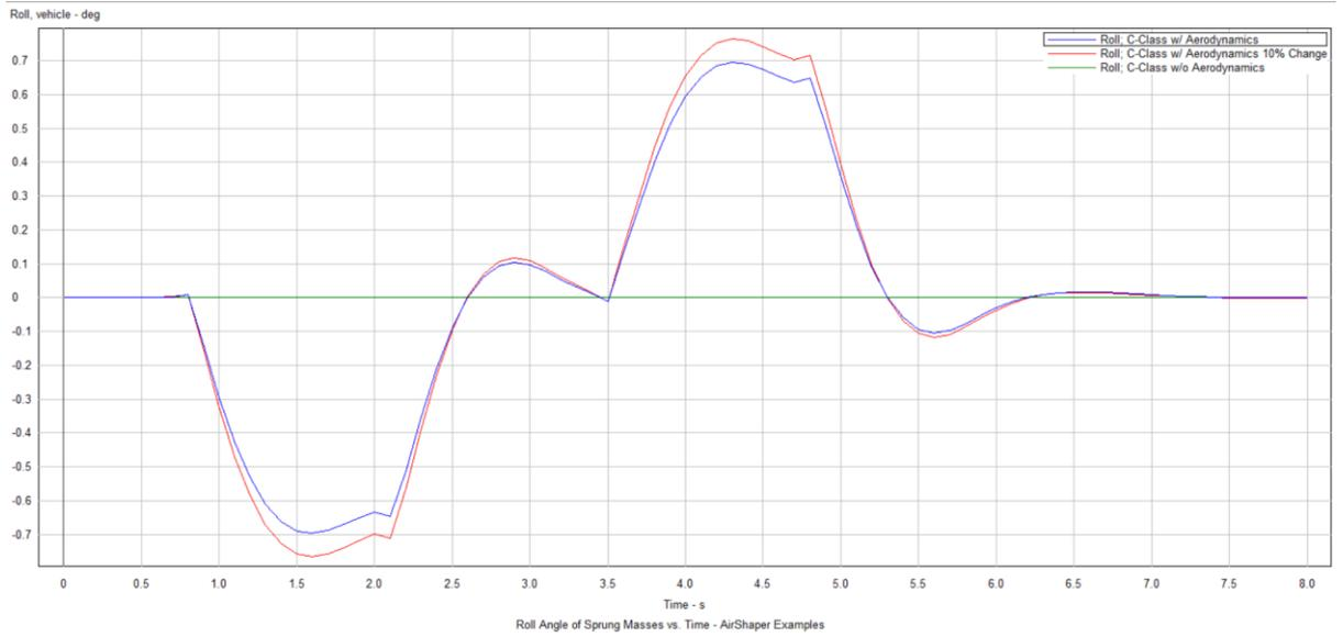
Figure 6: Roll angle variation due to Crosswinds all coefficients changed
