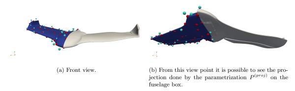
Figure 5: Reference geometry (blue) and a random configuration. Control points C (red) and deformed control points C + D (light blue).
