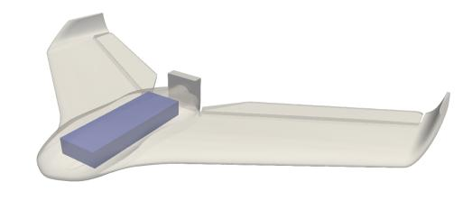
Figure 6: Physical space constraints handled by the projection parametrizer.
