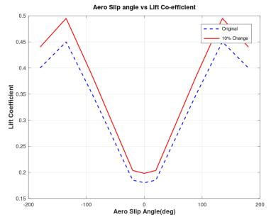
Figure 28: Lift Coefficient versus Aero Slip
