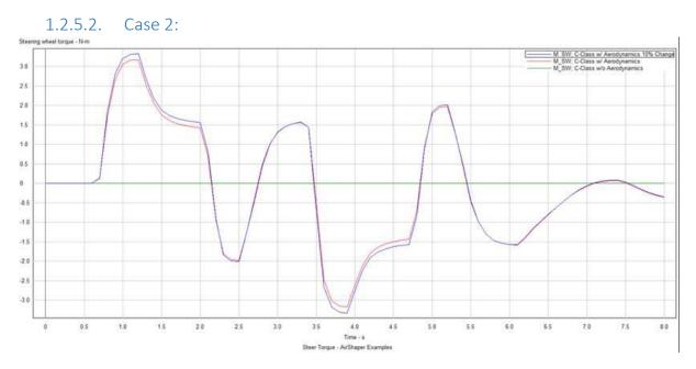
Figure 11: Steering Torque v/s time comparison crosswind <u>only lateral coefficients changed</u>
