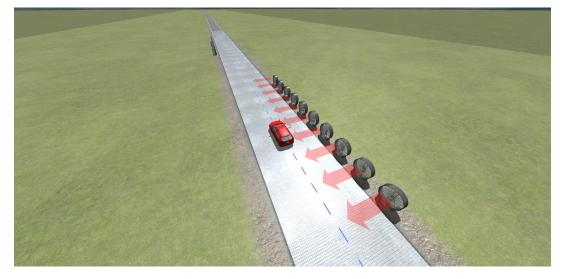
Figure 1: Crosswind Procedure setup
