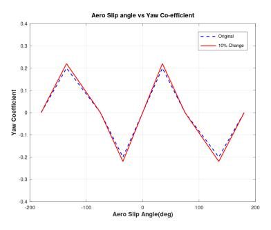
Figure 25: Yaw coefficient versus Aero Slip Angle
