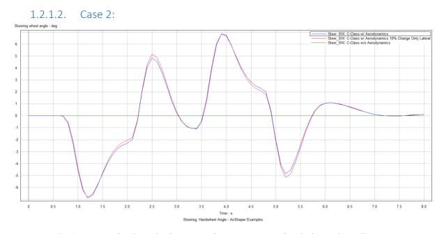
*Figure 3: Steering wheel angle deviation due to crosswind <u>only lateral coefficient</u> <u>changed</u>*
