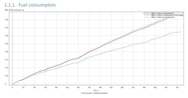
Figure 13: Fuel Consumed Over EPA Highway Cycle
