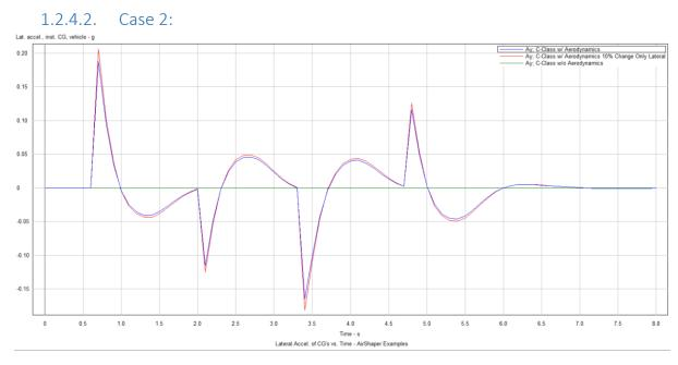
*Figure 9: Lateral Acceleration comparison crosswind <u>only lateral coefficients</u> <u>changed</u>*
