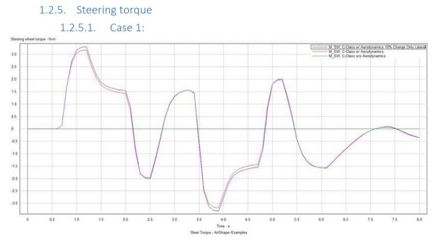
Figure 10: Steering Torque v/s time comparison crosswind <u>all co-efficient changed</u>
