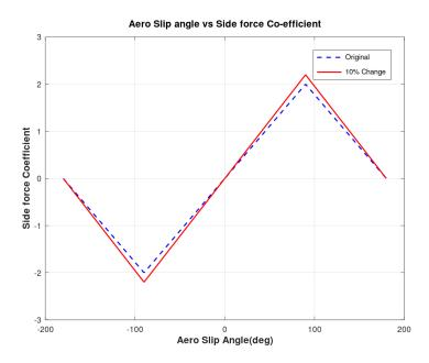
Figure 29: Side force coefficient versus Aero Slip
