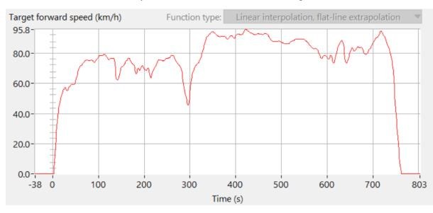
Figure 12: Vehicle Speed Profile EPA Highway Cycle
