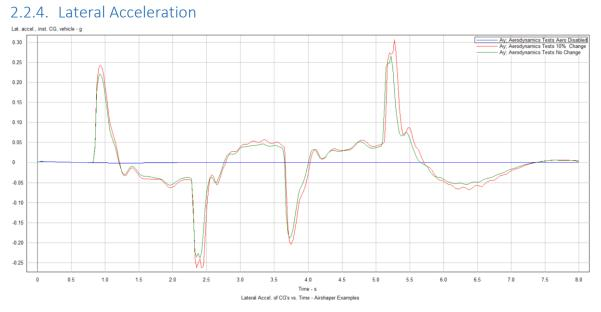
Figure 18 : Lateral acceleration versus time for different aero conditions
