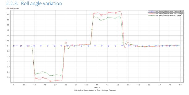
Figure 17: Roll angle versus time for different aero conditions
