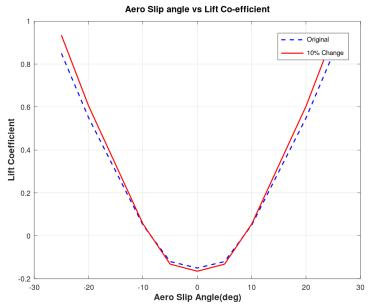
Figure 35: Aero Slip versus lift co-efficient
