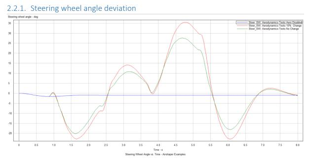
Figure 15: Steer angle versus time for different aero conditions
