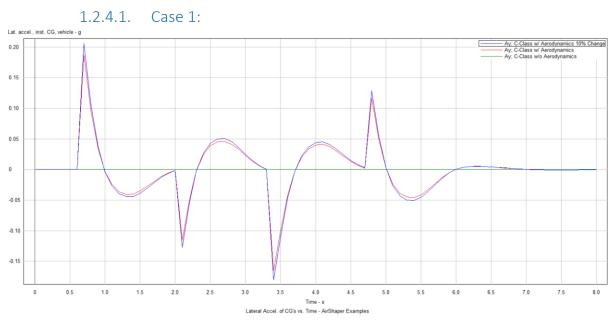
*Figure 8: Lateral Acceleration comparison crosswind <u>all co-efficient changed</u>*
