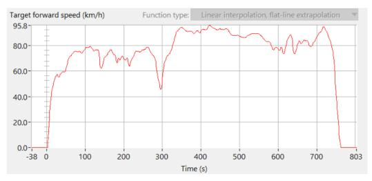
Figure 20: Vehicle Speed profile EPA Highway cycle
