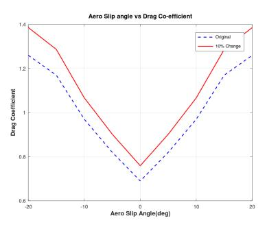
Figure 37: Aero Slip versus drag co-efficient
