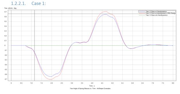
Figure 4: Yaw angle deviation due to crosswinds <u>all coefficients changed</u>
