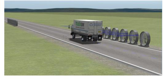
Figure 14: TruckSim Crosswind Simulation
