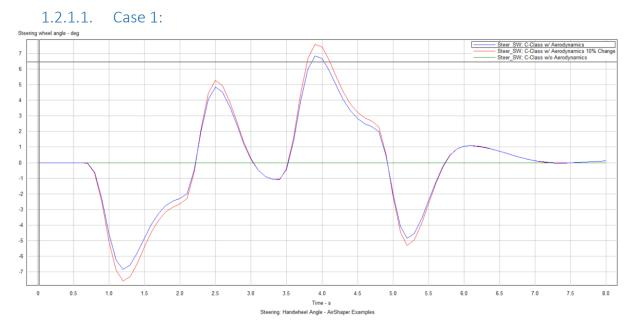
Figure 2: Steering wheel angle deviation due to crosswinds <u>all coefficients changed</u>
