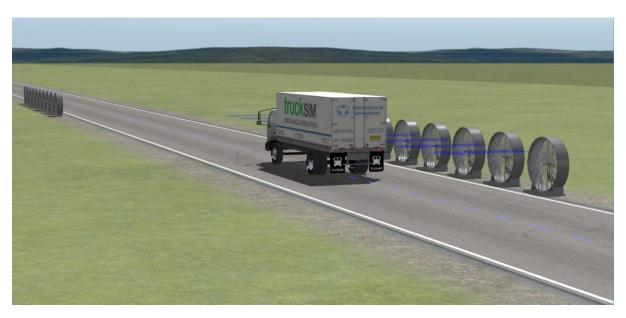
Figure 31: TruckSim Crosswind Simulation
