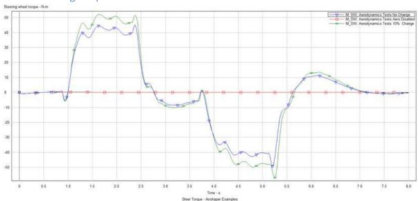
Figure 19 : Steering torque versus time for different aero conditions
