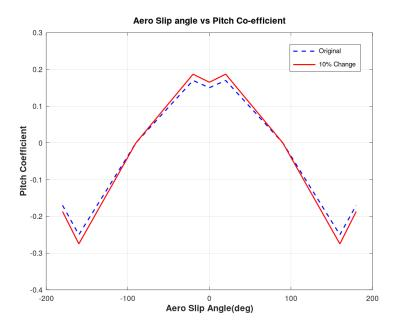
Figure 26: Pitch coefficient versus Aero Slip
