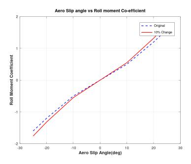
Figure 34 : Aero Slip versus roll moment co-efficient
