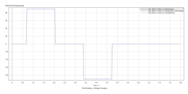
Figure 24: Crosswind heading angle input +90 deg & -90 deg
