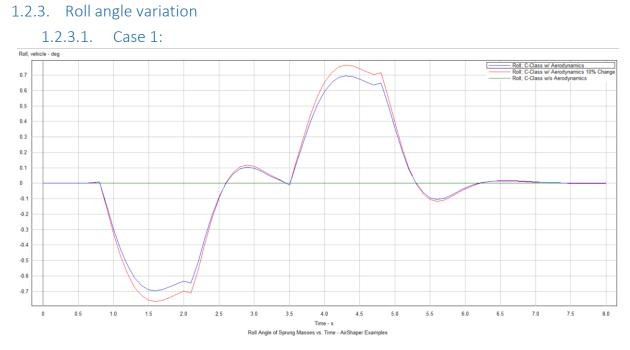
Figure 6: Roll angle variation due to Crosswinds all coefficients changed
